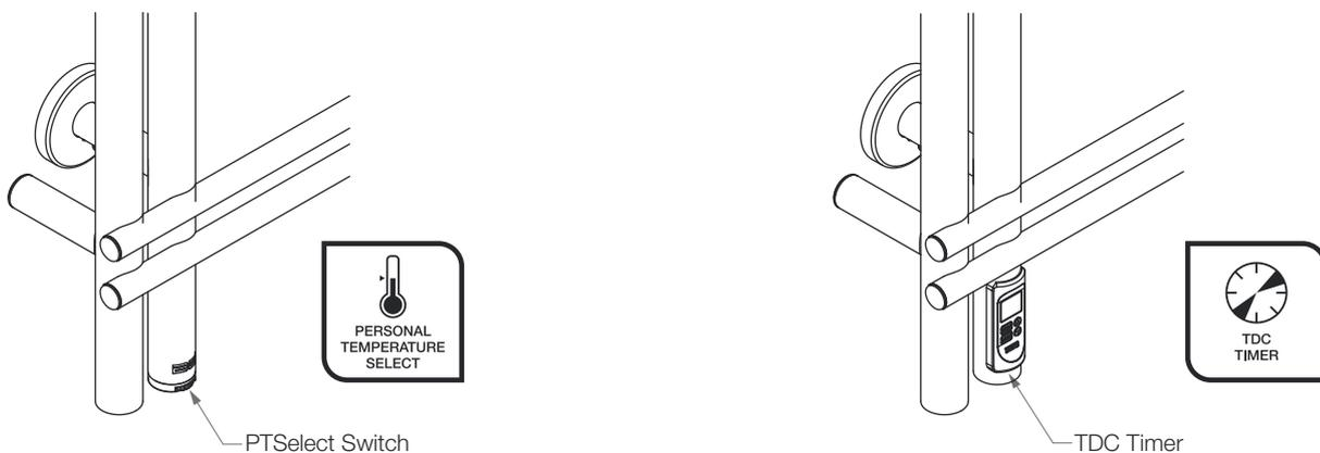
PTSelect Switch allows you to switch the HTR ON and OFF as well as adjust the temperature.
