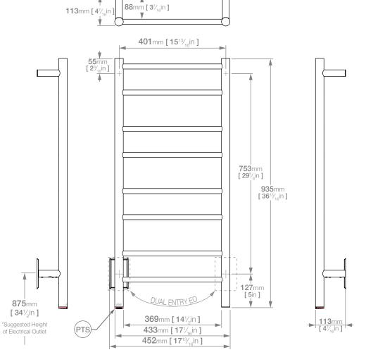
Dimensions given are in mm. Bathroom Butler® reserves the right to alter and/or remove designs from time to time without prior notice. This drawing is to be used for reference purposes only. E &O.E.
